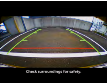
Rear view monitor A live color image with parking guidelines helps prevent backing into objects or other hazards out of sight.
