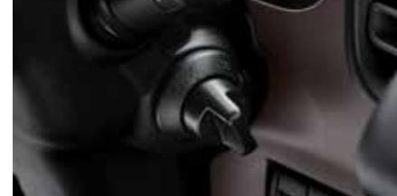
Keyless entry is available by simply pushing the lock/unlock switch on the door handle while the FUSO Easy Access Key is in a pocket or other location close by. The doors can also be locked/unlocked by operating the remote key near the vehicle. To start the motor, simply turn the starter switch on the steering column. This system is convenient for tasks like deliveries in the city that repeatedly involve getting in and out of the cab and frequent starting and stopping of the vehicle.
