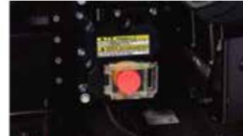
Do not press this switch except in an emergency. The High-voltage Cutoff Switch will not return on its own once it is depressed. The vehicle must be taken to a service shop to clear the diagnostic trouble code (DTC).
