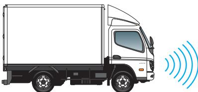
AVAS is a system for warning people outside the vehicle that the vehicle is approaching. It is not intended to prevent collisions. When driving, be sure to check the safety of your surroundings and drive safely.
